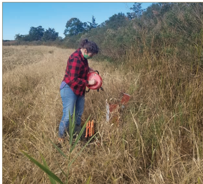
DGS staff member, Rachel McQuiggan, measuring water levels for the Delaware Groundwater Monitoring Network.
